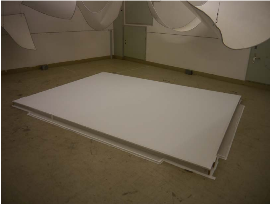
figure B1. test specimen in the reverberation room
